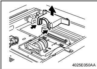
5. .Remove two hooks and the lens cover.
