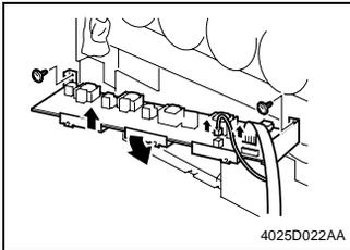
15. Disconnect the connectors and flat cable from the High Voltage Unit (Developing Bias).
