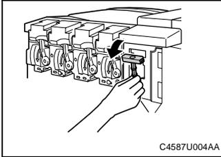
6. Remove the IU removal jig ("T" Handle) for the Imaging Unit from the Main unit.
