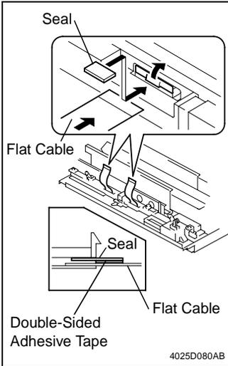
3. Insert the flat cable into the LPH Assy and lock the LPH Assy.
