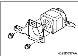
5. Remove two screws and the Scanner Motor.
