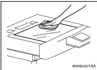
1. Using a soft cloth dampened with alcohol, wipe the Original Glass clean of dirt.
