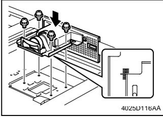
1. Align the CCD Unit with the center of the graduations as illustrated on the left and then tighten the four screws.
