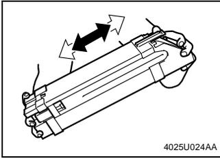
1. Remove the Imaging Unit from its aluminum pack.
