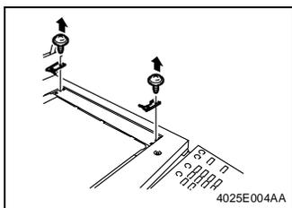
2. Remove one screw each and the Original Glass fixing bracket (at the front and rear).
