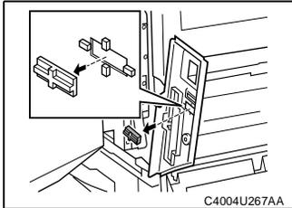
4. Cut out the knockout in the Front Right Cover.
