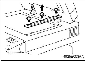
1. Remove three screws and the IR Right Cover.
