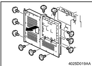
10. Remove 11 screws and lift the PWB box upward and off the copier.
