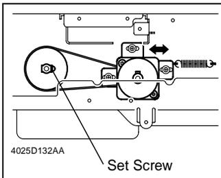
4. With the Scanner drive gear set screw located on the right-hand side as shown on the left, slide the Scanner Motor Assy to the left and check that it is returned to the original position by the tension of the spring. Perform this step three times.
