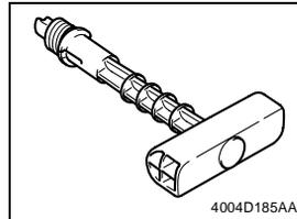
Imaging Unit Removal Jig
