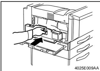
6. Clean the surface around the waste toner collecting port. [See (16) Cleaning of the Area around the Waste Toner Collecting Port.]
