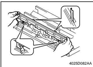
5. Holding onto both ends of the LPH Assy, align the portions shown on the left and then press it down into the locked position.
