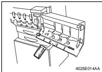
3. Remove the LED Cleaning Jig and LED Cleaning Jig Pad.
