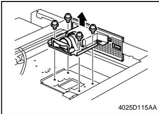
5. Remove four screws and the CCD Unit.
