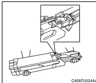
13. Insert the old Imaging Unit into the Imaging Unit Cover.
