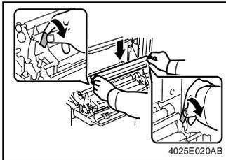
1. Holding onto the blue lock levers (at two places), mount the Image Transfer Roller Unit.
