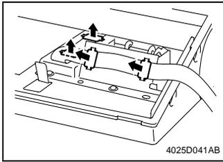
3. Remove the holding bracket and flat cable.
