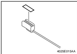
4. Affix a LED Cleaning Jig Pad to the LED Cleaning Jig.
