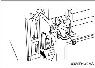
5. Remove two screws and unplug one connector on the PIC Board.
