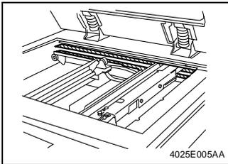
4. Using a soft cloth dampened with alcohol, wipe the Scanner Rails clean of dirt.
