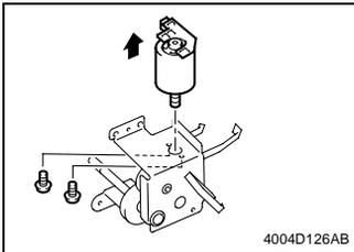
10. Remove two screws and the Fusing Pressure/Retraction Motor.
