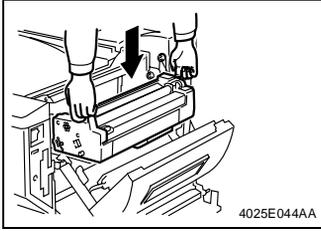
1. Hold the handles (at two places) and place the Fusing Unit in position.
