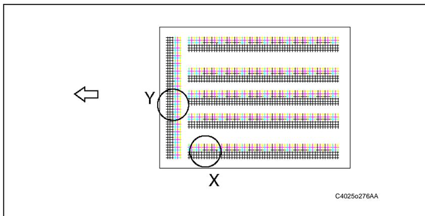
Adjustment for X direction: Check point X
