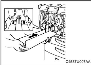
9. Position the Imaging Unit Pull-out Tray under the Imaging Unit and insert it all the way into position.
