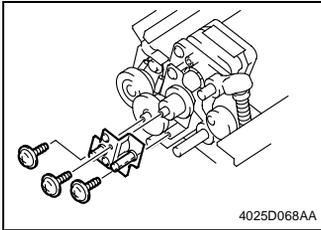
9. Remove three screws and the mounting bracket.
