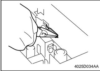
3. Remove the tension spring for the Scanner Motor timing belt.
