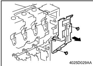
6. Remove two screws and the Front Door Switch cover.
