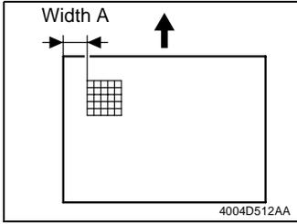
Width A on the test pattern produced should fall within the following range.
