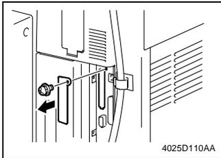
2. Remove one screw and the metal Blanking Plate.
