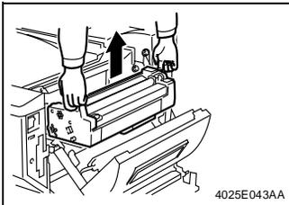
5. Hold the handles (at two places) and remove the Fusing Unit.
