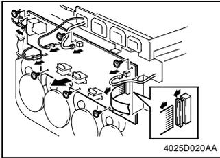
11. Disconnect connectors, terminals, and flat cable from the High Voltage Unit (Image Transfer, Neutralizing).
