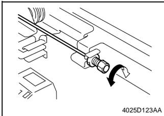
2. Turn the cable length adjusting screw so that the 2nd/3rd Mirrors Carriage contacts the cutouts in the rails.
