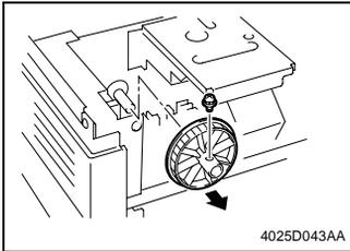
14. Remove one screw and the Scanner drive gear.
