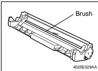
5. Turn over the Transfer Cleaner Assy so that the brush faces upward.
