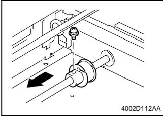
11. Remove the Scanner Motor Assy.
