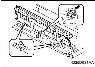
2. Unlock the LPH Assy and place the pivot tabs (at two places) at the upper position.
