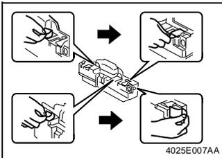
5. Peel off the seals for blocking the two toner collecting ports, and place them over the toner collecting ports.
