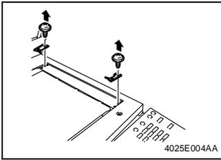
2. Remove one screw each and the Original Glass fixing bracket (at the front and rear).
