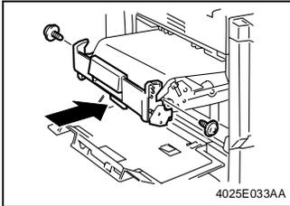
9. Fit bosses (at the front and rear) of the Transfer Cleaner Assy into the hooks (at the front and rear) of the Transfer Belt Unit.
