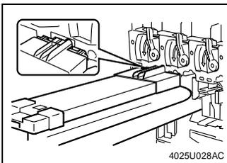
5. Keeping the Imaging Unit in a level position, insert the Imaging Unit into the mounting position all the way until it is stopped.
