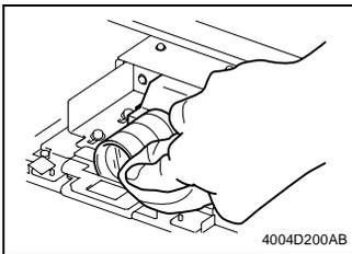
5. Using a soft cloth dampened with alcohol, wipe the Lens clean of dirt.
