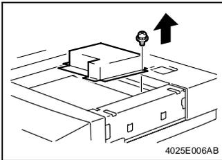
4. Remove fourteen screws and the optical cover.
