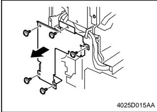
4. Remove five screws and the harness protective metal bracket.
