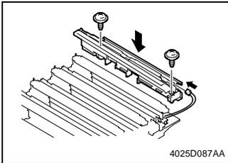
10. Install the two screws to secure the guide assy.
