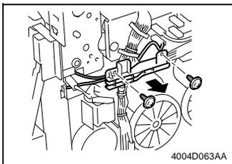
3. Remove two screws and the harness holder.
