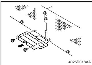
9. Remove two screws and the power line mounting bracket for the 2nd Drawer.
