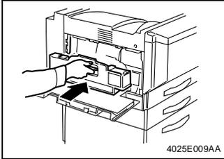
13. Hold the handle and install the Waste Toner Bottle in position.
