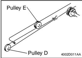
17. Wind the hook end of the cable around pulley D and pulley E.
