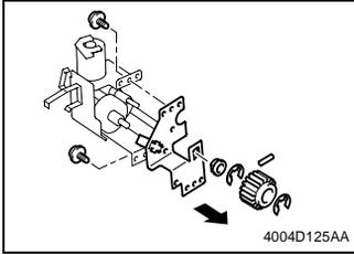
6. Snap off one E-ring and remove the gear and pin.
