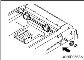
9. Install the front and rear pulleys and bushings onto the shaft and fit the C-clip.
