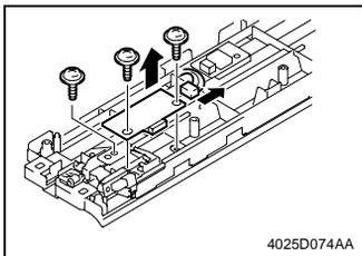
7. Remove three screws, unplug one connector, and remove AIDC/Registration Sensor 1.
