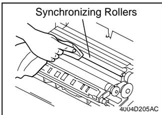
3. Using a soft cloth dampened with alcohol, wipe the Synchronizing Rollers clean of dirt.
