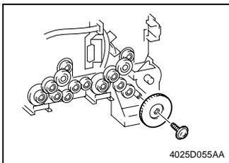
4. Remove one screw and the gear.
