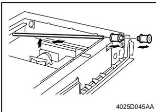
16. Slide the shaft toward the rear and lift it. Then, remove the front and rear pulleys.
