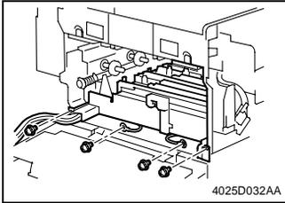
10. Remove four screws and slide out the LPH Unit.
