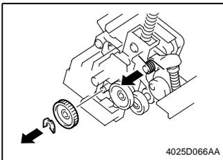
5. Snap off the C-clip and remove the gear.
