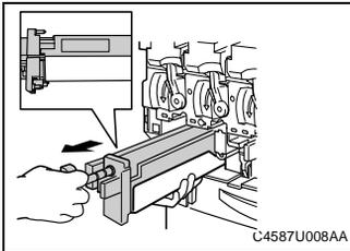
10. Supporting the Imaging Unit Pull-out Tray with one hand and holding the "T" Handle with the other, carefully slide the Imaging Unit out of the Main Unit. After removing the Imaging Unit place it on a level surface and cover it with a light blocking cloth.
