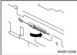
18. Fit the hook end of the cable to the spring and then hook the spring to the catch in the frame.
