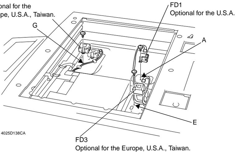
How the Harness should be Placed
