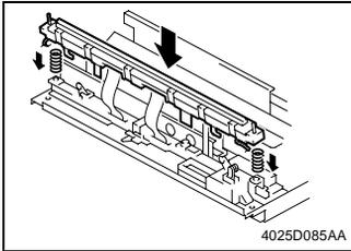
7. Hook the springs and press the LPH Assy down into the locked position.
