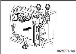
5. Remove three screws, unplug three connectors, and remove the rear left metal bracket.
