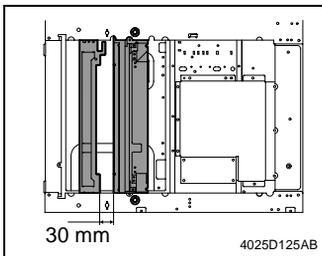
2. Secure the Scanner in the position shown on the left using Scanner positioning Screws.
