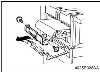
2. Supporting the Transfer Cleaner Assy with a hand, remove two screws.
