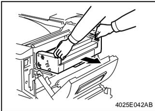
4. Hold the handles (at two places) and slide out the Fusing Unit.
