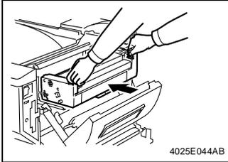
2. Hold the handles (at two places) and push the Fusing Unit into position.
