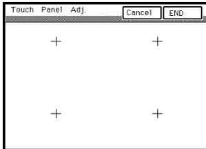
2. Using the tip of a pen or similar object, touch the four crosses (+) on the screen in sequence.
