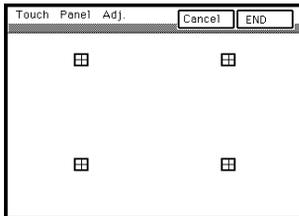
3. The cross touched changes into a grid marker that consists of a square with a cross superimposed.
