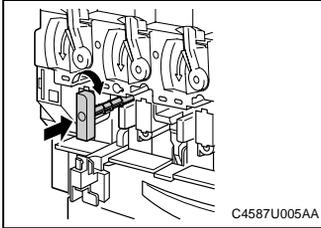
7. Set the removal jig of the Imaging Unit in place.
