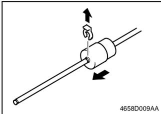
5. Snap off one C-clip and remove the Paper Take-Up Roller.
