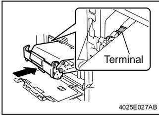
1. Insert the Transfer Belt Unit halfway up to the point shown on the left.
