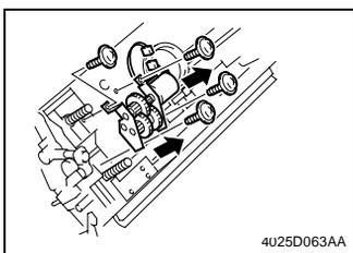
3. Remove four screws, unplug one connector, and remove the gear assy and motor assy.
