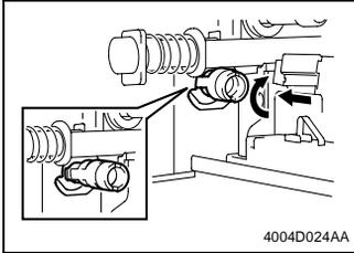
8. Open the Right Door and Left Door and remove the Waste Toner Bottle and Transfer Belt Unit.
