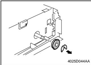
15. Snap off the C-clip and remove the bushing (front).
