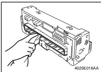
1. Remove the Fusing Unit.
