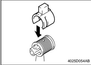
8. Slip the Cable Holding Jig onto the pulley to secure the cable in position.
