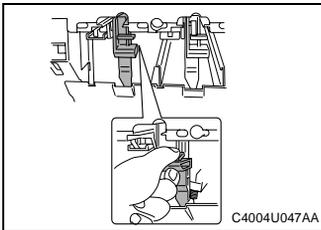
5. Release the lock lever of the Imaging Unit.
