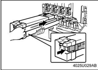
6. Holding the underside of the Imaging Unit with your left hand, gently insert the Imaging Unit with your right hand.
