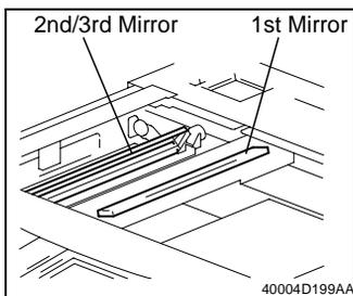
4. Using a soft cloth dampened with alcohol, wipe mirrors clean of dirt.
