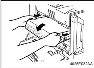
8. Holding onto both ends of the Transfer Belt, rotate the Transfer Belt until the Blade of the Transfer Cleaner Assy contacts the location on the belt, to which the toner has been applied.
