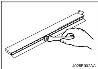
3. Using a brush, whisk dust off the Paper Dust Remover.
