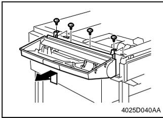
4. Remove four screws and the control panel base.
