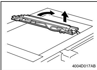
3. Take out the Scanner Assy by turning it in the direction of the arrow shown.
