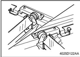
1. Slide the 2nd/3rd Mirrors Carriage to the center until it is pressed up against the cutouts in the rails.
