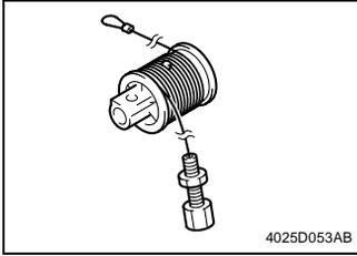
7. Wind the hook end of the cable around the pulley five turns counterclockwise, from the rear toward the front side.
