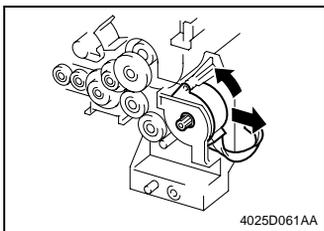
5. Remove two screws. Then, turn the Toner Replenishing Motor Y/M counterclockwise and take it off the copier.
