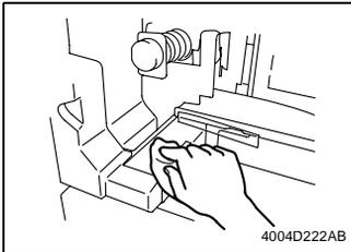
3. Wipe the areas around the Waste Toner Collecting Port clean of spilled toner and dirt using a soft cloth dampened with water or alcohol.
