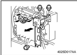
5. Remove three screws and unplug three connectors. Then, remove the rear left metal bracket.
