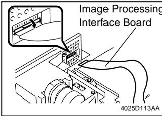
3. Remove the Image Processing Interface Board cable from the CCD Unit.
