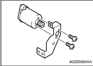
4. Remove two screws and the 2nd Image Transfer Pressure/Retraction Motor.
