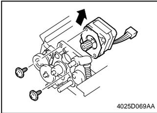
10. Remove two screws and the Transport Roller Motor.
