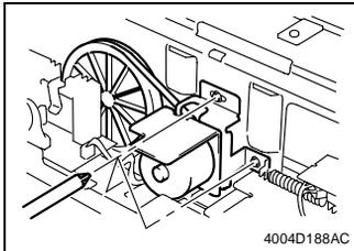
3. Loosen the three screws that secure the Scanner Motor mounting bracket.
