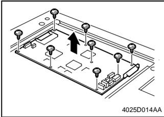
9. Remove eight screws and the Image processing Board.
