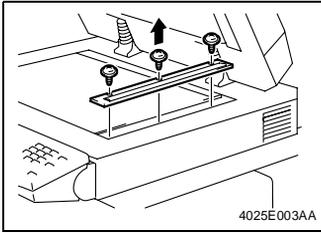
1. Remove three screws and the IR Right Cover.
