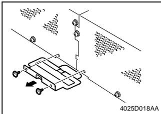
9. Remove two screws and the 2nd Drawer power line mounting bracket.
