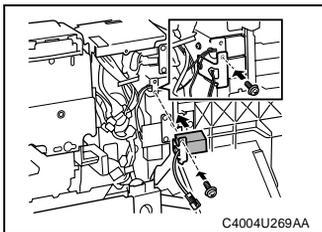
6. Secure the mechanical counter with one screw.
