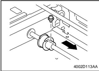
13. Remove one screw and then slide the rear pulley toward the front.
