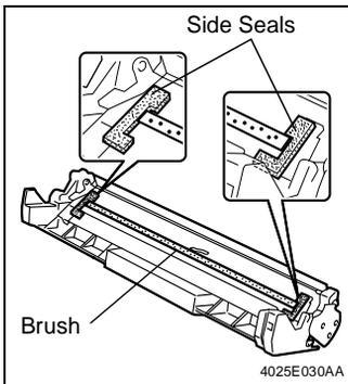
6. Uniformly apply the enclosed toner along the brush and on the side seals.
