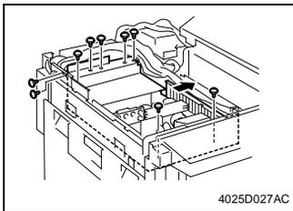
5. Remove nine screws and slide DC Power Supply 1 to the right.
