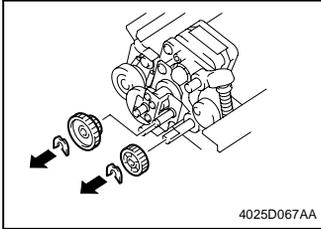
8. Snap off the C-clip and remove two Gears.
