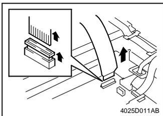
5. Remove the Image Processing Interface Board cable.
