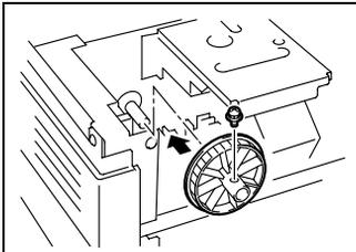
10. Mount the Scanner drive gear on the shaft and secure it using one screw.
