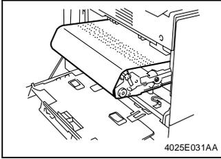
7. Place the remainder toner on the paper towel that comes with the Transfer Belt Unit and apply an even coat of toner on the Transfer Belt (up to 15 mm from both edges).
