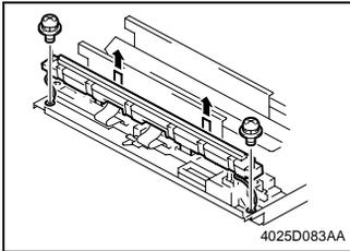
8. Remove the LPH Assy mounting jigs.
