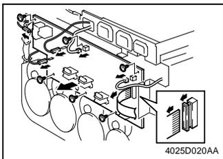
3. Disconnect connectors, terminals, and flat cable.
