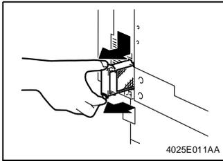
1. Holding onto the hook, remove the Ozone Filter.
