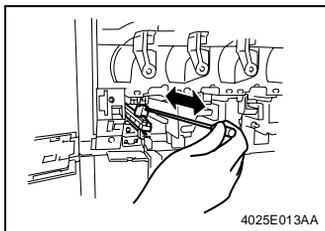
5. Clean the LED of the LPH Assy by moving the LED Cleaning Jig three reciprocating motions.
