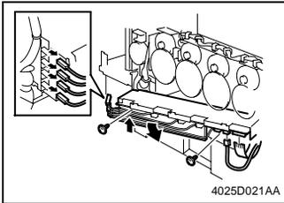
13. Disconnect connectors, terminals, and flat cable from the High Voltage Unit (PC Drum CH.).
