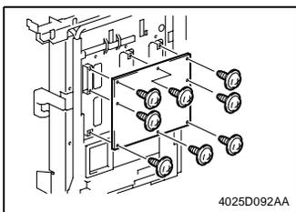
4. Remove eight screws, unplug two connectors, and remove the LED Drive Board.
