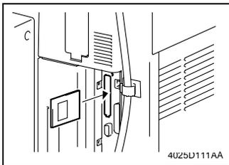
3. Insert the memory card into the slot.
