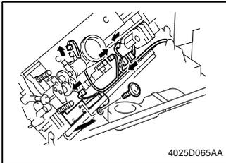
3. Remove one screw, ground wire, and ground plate.
