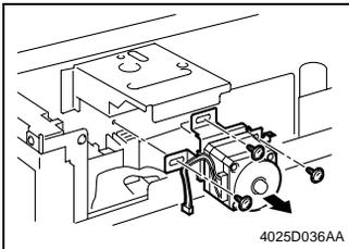
4. Remove three screws and the Scanner Motor Assy.
