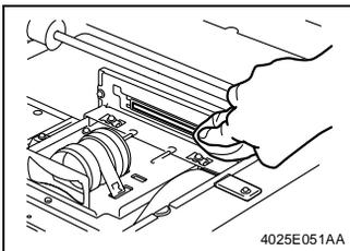
6. Using a soft lint free cloth dampened with alcohol, wipe the CCD Sensor clean of dirt.
