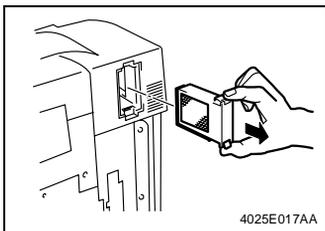
1. Holding onto the hook, take out the Deodorant Filter.
