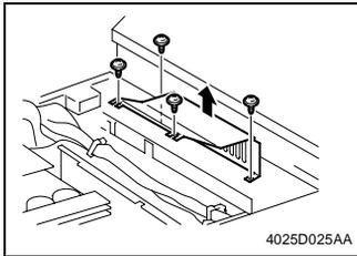
3. Remove four screws and the PWB cover.
